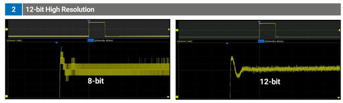
12-bit resolution shows you more details and less noise on the waveform.
