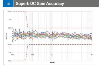
Low noise floor: Only 70 μVrms at 200 MHz bandwidth 0.5 % DC gain accuracy
